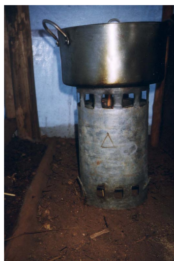
Peko Pe metal stove (the outer cylinder and the combustion chamber plus its ring cover are built from iron sheeting)
