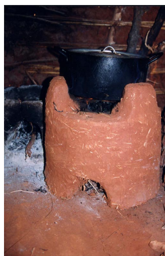
Peko Pe clay-metal stove (the outer cylinder is built from a clay-soil mixture and only the combustion chamber and its ring cover are built from iron sheeting)
